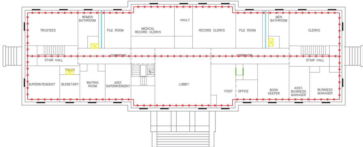
2 ASBESTOS CONTAINING THERMAL SYSTEM INSULATION MATERIALS LOCATION FIRST FLOOR – NEWTOWN HALL SCALE: 3/32"= 1'-0"
