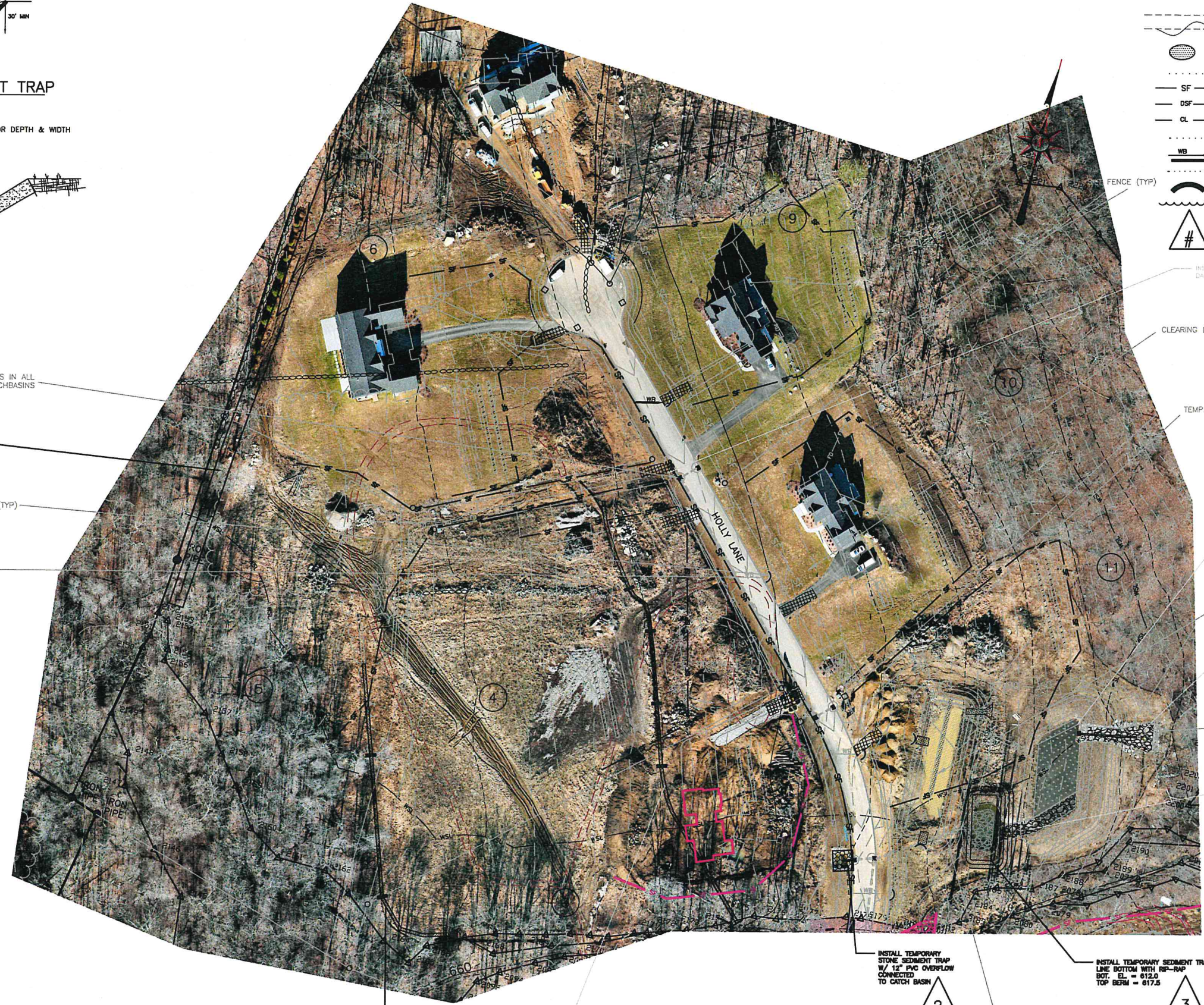
SEDIMENT TRAP #2 BOTTOM ELEV=617.0 AREA=4,300sf BOTTOM DIKE=620.0 AREA=5,800sf SPILLWAY=622.0 AREA=7,200sf TOP BERM=623.0
